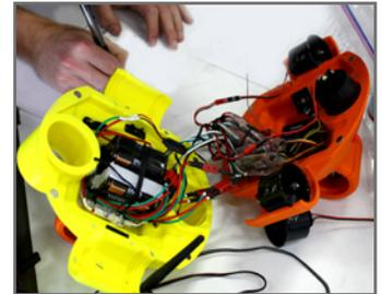
Top shell (yellow) and bottom shell (orange) are both FDM parts.
