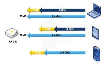
Enhanced receive sensitivity also has the added benefit of making 5Ghz coverage much broader and available to more clients who support the 5Ghz band, which helps to free up the over-used and crowded 2.4Ghz spectrum and allows higher speed radio communication on both spectrums. All in all, more intelligent access points combined with cloud-managed, cooperative control software enhance the Wi-Fi experience on any type of device, consumer-focused or not.
