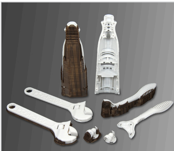
3D-printed models are shown with soluble support material (brown) intact, and after removal.
