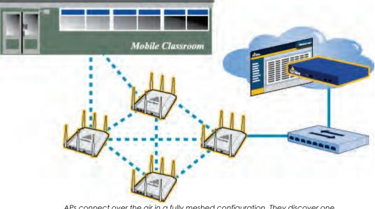
APs connect over the air in a fully meshed configuration. They discover one another, route around failures, and forward traffic to each other using the best path available. An AP can be added in a portable classroom or elsewhere and removed without any ramifications to the infrastructure.
